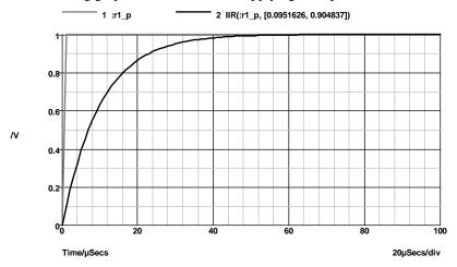
The coefficients used give a time constant of 10 \* the sample interval. In the above the sample interval was  $1\mu Sec$  so giving a  $10\mu Sec$  time constant. As can be seen a first order IIR filter has exactly the same response as an single pole RC network. A general first order function is:
