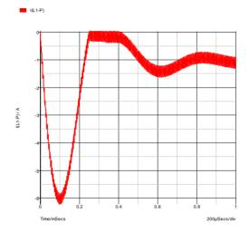
This shows that the operating current is less than 1.5A but peaks at over 6A. In practice you would want to use an inductor with a maximum current of around 2A in this application; an inductor with a 6A rating would not be cost-effective. We will now replace the ideal component, with something closer to a real inductor.
