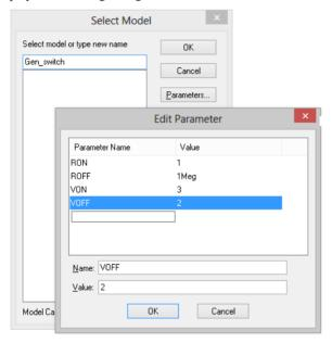
If On Voltage > Off Voltage If control voltage > On Voltage Resistance += On Resistance else if control voltage < Off Voltage Resistance = Off Resistance
