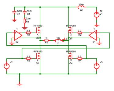
Sources V2 and V3 have been defined to be dependent on a parameter named duty which specifies the duty cycle of the switching waveform. See Examples\Spice\Bridge\Bridge.sxsch.
