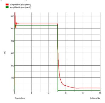
The green trace(the cleaner of the two) is the output after the modification. As you can see, the problem with the trailing edge has been fixed and the ringing is much improved.
