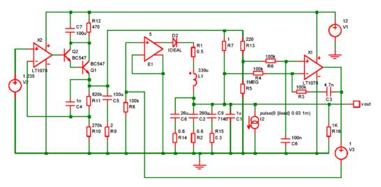
12 provides a current that is switched on for 1mS after a short delay. A multi-step analysis is set up so that the load current is varied from 10mA to 1A. The output for all runs is:
