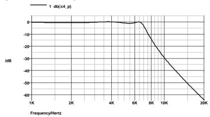
This circuit is to be used in an application that requires the gain of the amplifier to remain within 2dB of the dc value from 0 to 6kHz. A 1dB ripple specification therefore seems a reasonable choice. Clearly though the tolerance of the capacitors and resistors may upset this. To investigate, a Monte Carlo analysis is required. The standard component tolerances are 10% for capacitors and 1% for resistors. To apply these tolerances, proceed as follows.
