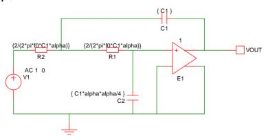
The above circuit is that of a two pole low-pass filter. C1 is fixed and R1=R2. The design equations are:
