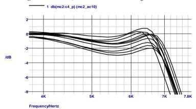
As can be seen, the specification is not met for some runs. Note that - as a rule of thumb - the spread for 10 runs will be about half of a realistic maximum spread  $(3\sigma)$ .
