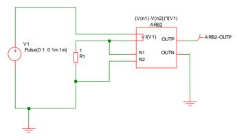
In the above, ARB2 is the device created from the Non-linear Transfer Function menu. ARB2-OUTP will carry a voltage equal to the power dissipation in R1.
