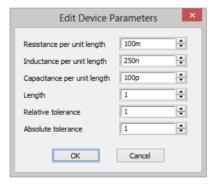
Lossy lines must be defined in terms of their per unit length impedance characteristics. Currently only series losses are supported.
