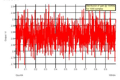
The graph shows the variation in gain for 1000 samples. Using the histogram feature a statistical distribution of the above can easily be plotted.
