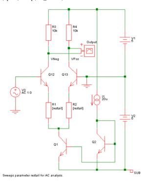
This is a simple long tailed pair. The above circuit resistors R1 and R2 have been given the values {restail}. *restail* is a parameter that is swept in an AC sweep to plot the gain of the amplifier vs tail resistance at 100kHz. Here is the result of the run:
