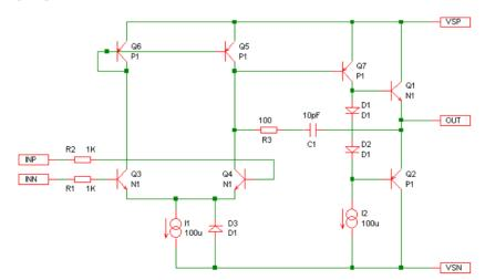
The five rectangular **Subcircuit Pin** components are the connections to the outside world.
