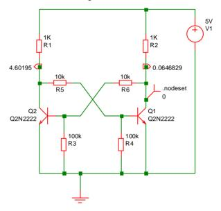
A nodeset has been applied to the collector of Q1. This has forced Q1 to be on and Q2 to be off. If the nodeset were absent the solution would actually leave both Q1 and Q2 partially on. In real life this would not be stable but is numerically accurate.
