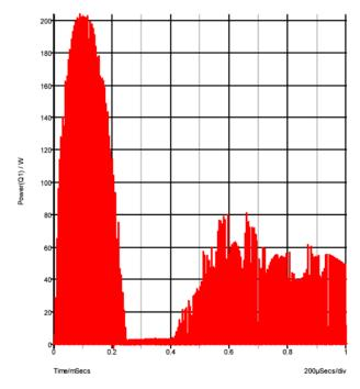
8. This shows a peak power dissipation of 200W although you are probably more interested in the average power dissipation over a specified time.
