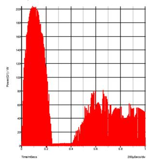
This shows a peak power dissipation of 200W although you are probably more interested in the average power dissipation over a specified time.
