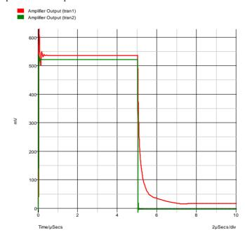
The green trace(the cleaner of the two) is the output after the modification. As you can see, the problem with the trailing edge has been fixed and the ringing is much improved.
