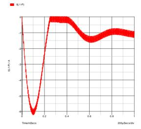
This shows that the operating current is less than 1.5A but peaks at over 6A. In practice you would want to use an inductor with a maximum current of around 2A in this application; an inductor with a 6A rating would not be cost-effective. We will now replace the component, with something closer to a real inductor.
