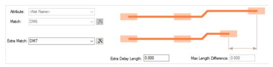
When the **Extra Match** rule is set to zero, this means simply ensure that the explicit nets are matched using the Max Length Difference. If, however, an explicit override rule is required, then the **Extra Delay Length** can be assigned (see below).
