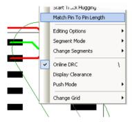
When matching lengths the head-up display will change to show the names of the pins we are trying to match, the length of the tracks between them, and the difference in lengths. The difference will be shown in the illegal colour if not zero.
