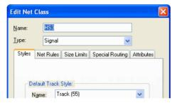
Routing now becomes Special Routing (this contains Serpentine Rules etc.). Rules becomes Net Rules but is also modified to include the new changes. Size Limits has been added for Version 7.0.
