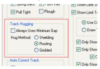
Shielding adds tracks that hug the obstacles as tight as possible, introducing arcs around pads and sharp corners (see below). This can be used to create shielding around tracks and other copper obstacles for RF protection for example.
