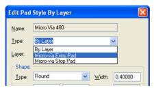
Normally, you would also do the same for the **Stop Pad** so the laser knows where to start and where to stop drilling, although this isn't mandatory for some processes. The Stop pad is displayed as a solid pad even though the default pad stack is defined with a drill hole, and the Entry pad is displayed with a drill hole shown (depending on Layer Class settings).
