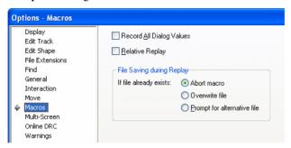
If **Relative Replay** is enabled and **Run Macro** is invoked while the mouse cursor is outside the design window, such as when selecting the Relative Replay option from the menu or toolbar, you are required to set the relative start position for the macro, using the mouse, before it will run. You will also see that the cursor has changed and is now a model cursor to indicate that a relative reference point is required.
