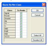
By using the **To Route** switch, net classes can be selected or deselected for use.
