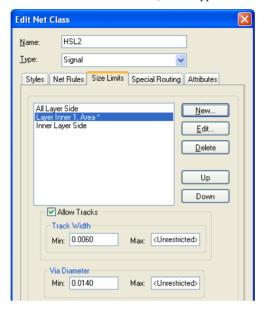
These rules are applied in the order defined in this list, until the first match is found. You should therefore have the more specific rules (in terms of layer, area and sub-net) defined at the top of the list. You can move a rule up and down the list by selecting the rule in the list and using the Up and Down buttons.
