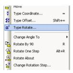
Use this to rotate the current selection about a particular point and by a specified amount by typing the values into a dialog.
