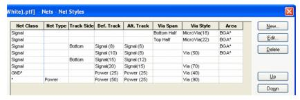
When adding a new track or via to the design, the style to be used is searched for through the **Net Styles** entries defined in the design, in the order defined in this dialog. The search will continue until a match is found taking into consideration the net class name, track layer side, via layer span and an area name (if within a styles override area).
