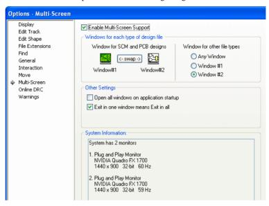
Select the **Enable Multi-Screen Support** check box to turn on this operation. With this enabled, two instances of the application will work together to arrange your files so you can easily work on Schematic designs on one screen, and PCB designs on the other. Each instance will have its own menus and toolbars and work independently, but will share information when they need to.
