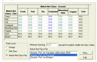
In this dialog, set the Rule Level to Match Net Class Rule and use the New button to define the area based rule. You will be presented with the Class To Class Rule dialog to setup the conditions for the spacing set to be used. Add the names of the net classes between which the spacings will apply, using wildcards to specify groups of net classes.
