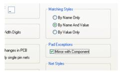
When checked, any pad style layer exceptions used on pads in mirrored Components will have their layer swapped to the other side. This was added specifically for Through-hole pad stacks where Top side or Bottom side pad stacks were defined. Surface Mounted pad stacks are left unaffected.
