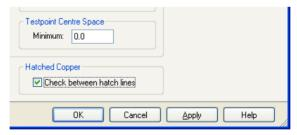
With this check box selected, the error reported is Net Split/Incomplete (N) when the item falls inside the Hatch area and is on the same net but not connected.
