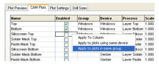
You can create a plot using the CAM Plot Wizard and add the plot to the Plot Group. Either select an existing plot group name from the drop down list or type a name in.
