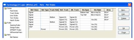
Use this page to build up an ordered list of default track and via styles with conditions based on net class name, area name track side and layer span.
