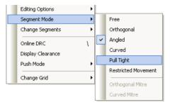
When routing in tight areas of the design, this can quickly produce results which are very space-efficient. This mode will 'wrap' tracks around obstacles and pull the result tight to
