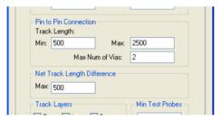
Nets using the net class with this rule will be checked when using the DRC option, Nets and **Track Length** options selected. If an error exists, an NLD error marker will be displayed. A more verbose error message will be shown in the Properties dialog of the relevant error marker.
