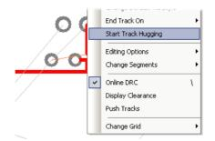
3. Right click the mouse and use **Start Track Hugging** from the shortcut menu. A better way to do this is to put the **Track Hugging** command onto a shortcut key and press the key when the cursor is over the track to hug.
