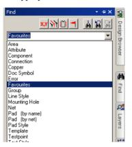
There are three small icons along the top of this window, (moving left to right) these indicate a drop down shortcut menu (also available as a shortcut menu in the window by right clicking the mouse), a pin to enable the dialog to be sliding to conceal it or docked to be permanently displayed, and a **Close** button to dismiss the dialog altogether.
