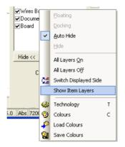
When the option is chosen, the layers on which the selected item resides will be switched on and all other layers switched off. This is also available as a command for assigning to a shortcut key.
