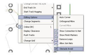
In obstacle avoid mode you can automatically remove any corners that have been added by retracing the cursor back over the track (like in auto corner).
